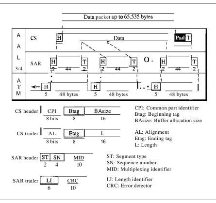
The CS layer header and trailer consist of six fields:
