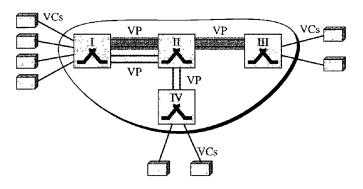
Identifiers In a virtual circuit network, to route data from one endpoint to another, the virtual connections need to be identified. For this purpose, the designers of ATM created a hierarchical identifier with two levels: a virtual path identifier (VPI) and a virtual-circuit identifier (Vel). The VPI defines the specific VP, and the Vel defines a particular VC inside the VP. The VPI is the same for all virtual connections that are bundled (logically) into one VP.
