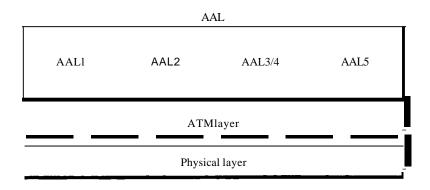
Figure 18.17 ATM layers in endpoint devices and switches
