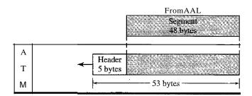
Header Format ATM uses two fonnats for this header, one for user-to-network interface (UNI) cells and another for network-to-network interface (NNI) cells. Figure 18.19 shows these headers in the byte-by-byte format preferred by the ITU-T (each row represents a byte).
